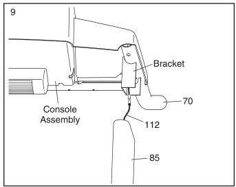
Attach the console assembly to the Uprights (85) with four Console Bolts (72) and four 3/8" Star Washers (67) (only one side is shown).
